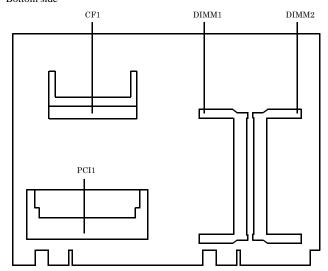
Figure 2.1. Connector & Jumper Location
